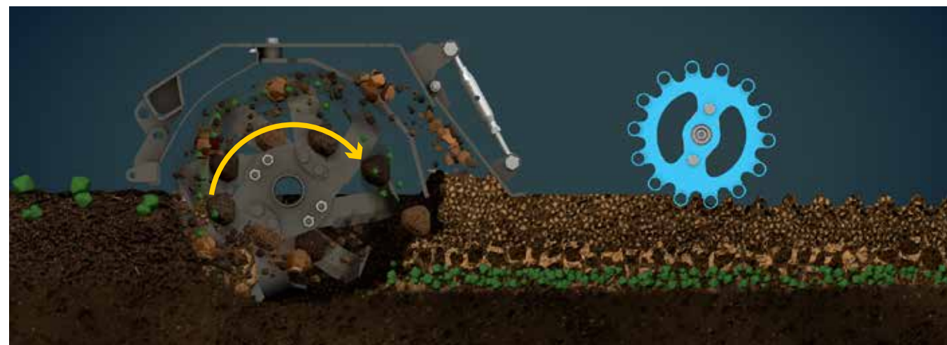
▲ Working of the overtop rotavator, the rotavator which turns against the direction of travel. Residue is milled in.
