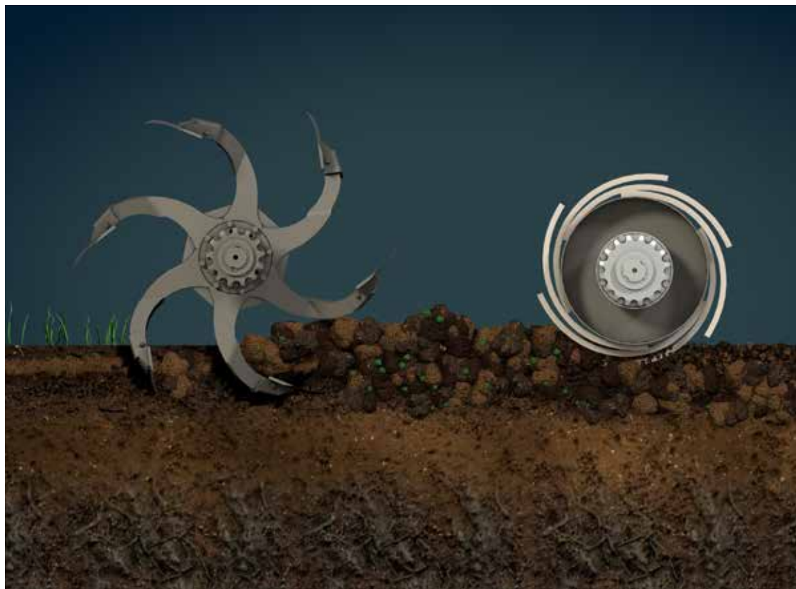
Spading shaft with power harrow
